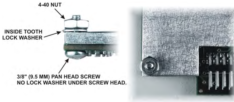
Figure 72 Stiffener Fastener on KSYN3 Board.
